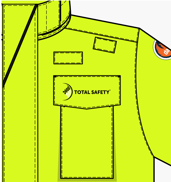
Company logo S0266 Heat transfer seal On chest pocket flap LHS Color: according to artwork Size: 100 x 36mm
