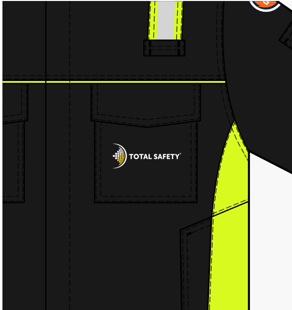
Company logo S0114 Heat transfer seal On chest pocket LHS Color: according to artwork Size: 100 x 36mm
